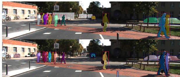
Fig. 1. Ground truth image ( top ) with ignored regions (white) and instance segmentation ( bottom ). The bounding boxes drawn around the instances represent the class, blue denotes cars and red pedestrians.
