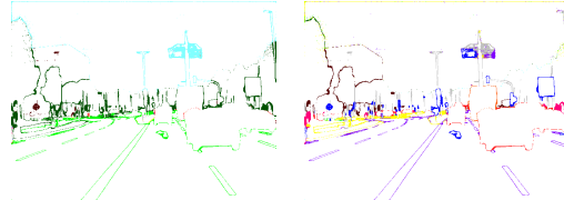
Figure 7: Visualization of the differences between the segmentations obtained from Bayes and ML. In both images the predictions differ mostly at the object boundaries, i.e., at the transition from one class to another. Left: The points in the Bayes prediction where Bayes and ML disagree. Right: The points in the ML prediction where Bayes and ML disagree.
