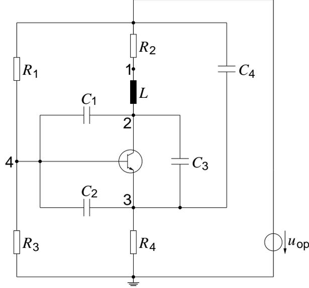
Fig. 5. Circuit of Colpitts oscillator.
