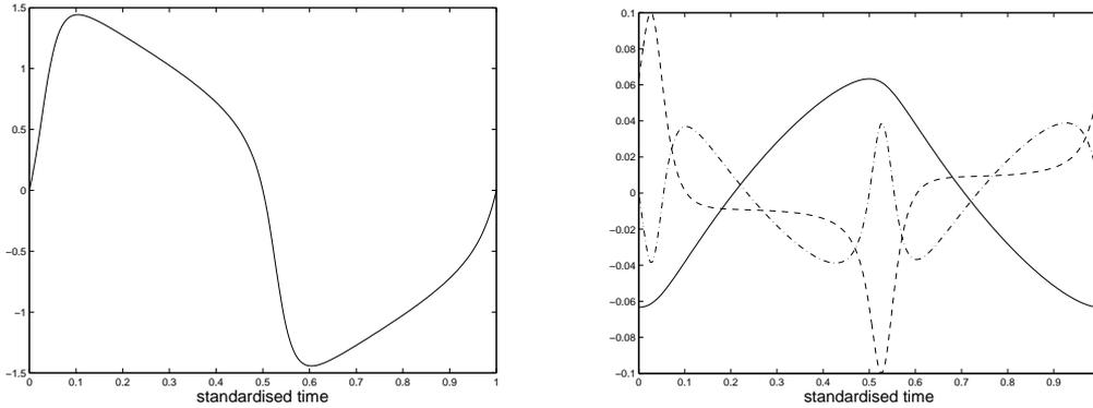
Fig. 2. Expected values of the node voltage (left) and the three branch currents (right,  $i_L$ : —,  $i_C$ : - - -,  $i_R$ : -·-·-) in VCO.
