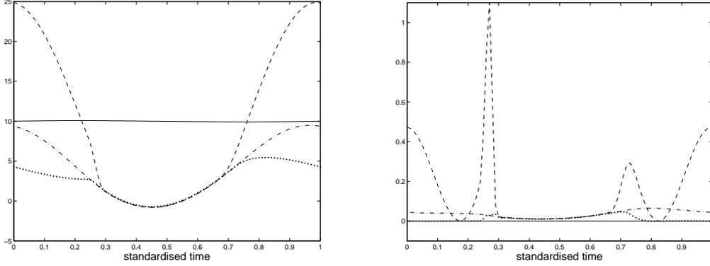
Fig. 6. Expected values (left) and variances (right) of node voltages in Colpitts oscillator ( $u_1$ : —,  $u_2$ : - - -,  $u_3$ : -·-·-,  $u_4$ : ···).
