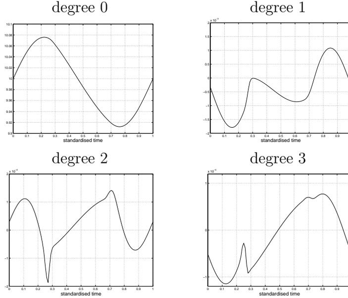
Fig. 7. Coefficient functions in gPC expansion of node voltage  $u_1$  in Colpitts oscillator.
