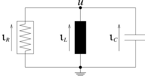
Fig. 1. Circuit of voltage controlled oscillator.
