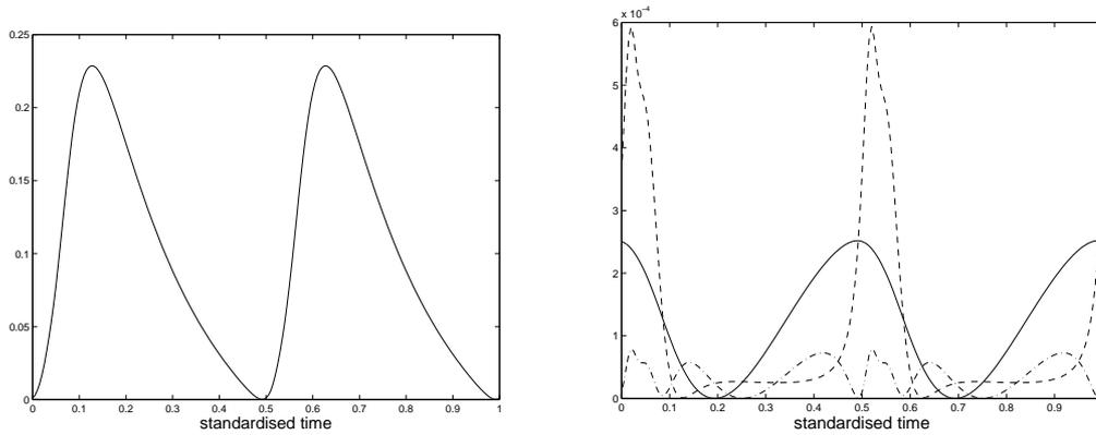
Fig. 3. Variances of the involved node voltage (left) and the three branch currents (right,  $i_L$ : —,  $i_C$ : - - -,  $i_R$ : - · - ·) in VCO.
