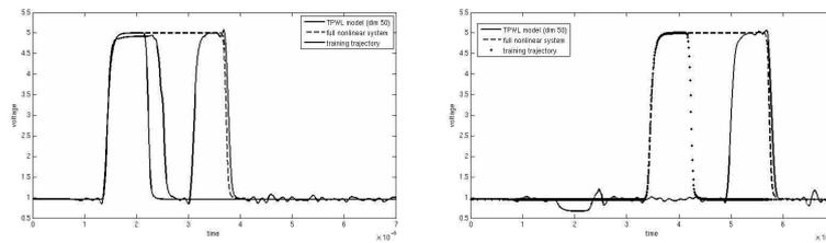
**Fig. 6** Inverter chain: TPWL-resimulation, reduction to order 50, wider pulse, distance in full space, Left: inverter 18; Right: inverter 68.
