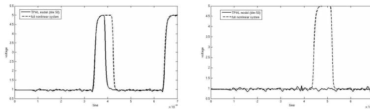
**Fig. 5** Inverter chain: TPWL-resimulation, reduction to order 50, repeated pulse, distance in full space, Left: inverter 68; Right: inverter 92.
