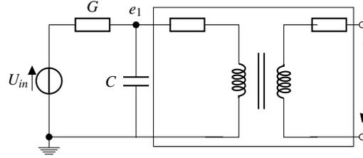
the circuit while the slow subsystem the electromagnetic effects of the transformer. Figure 1 shows a circuit diagram of the coupled system, the electromagnetic effects are represented by the lumped devices of a transformer in the box. The input voltage is given by a superposed sinus function  $U_{in}(t) = 45.5 \cdot 10^3 \sin(900\pi t) + 10^3 \sin(45000\pi t)$ .
