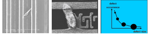
Fig. 1. Examples of disturbing bridges. Connections with small resistor values can lead to large defects to the solution.
