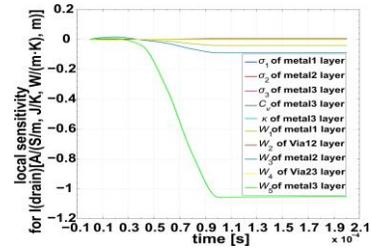
Fig. 4. Local sensitivity analysis of  $I(\text{drain})$  versus chosen parameter  $\mathbf{p}(\xi)$ .
