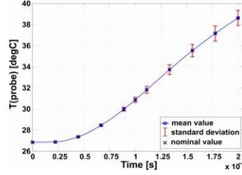
Fig. 3. UQ of  $T(\text{probe})$  due to variations of  $\sigma$  in Metal3, modeled by a uniform distribution with 15% variation around a mean 20 MS/m.
