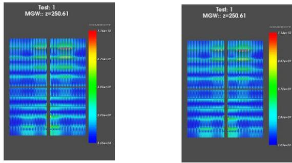
Fig.8. CD in Contact Layer after optimization: (left) DRO, (right) RTO.
