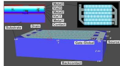
Fig. 1. Structure in a power transistor device [11].
