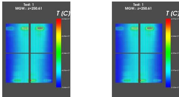
Fig.9. Distribution of T in optimized models: (left) the DTO, (right) the RTO.
