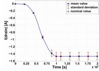
Fig. 2. UQ of  $I(\text{drain})$  due to variations of the Metal3 thickness, modeled by a Gaussian distribution with 10% variation around a mean of  $1 \mu\text{m}$ .
