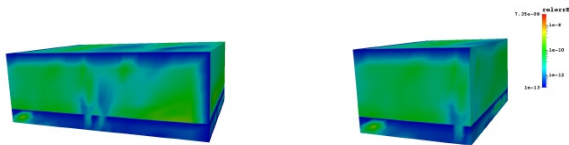
Figure 9: Relative error of the expectation of the electrical field in a coplanar waveguide.
