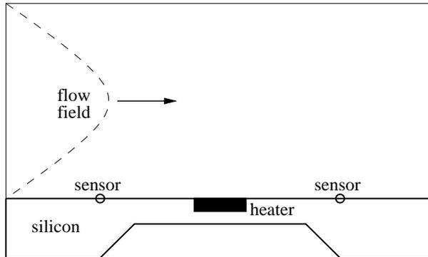
Figure 1: Layout of the anemometer.
