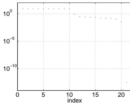
Figure 8: Singular values appearing in pMOR of RLC circuit.
