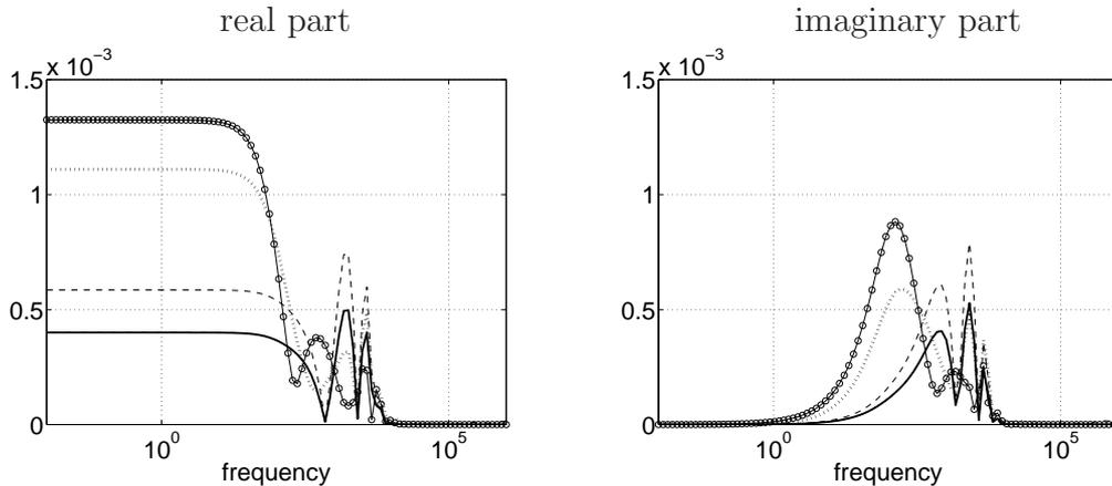
Figure 3: Standard deviation of the transfer function for the anemometer: reference solution (solid), MOR after SG (dashed), matrix sampling (dash-dotted), pMOR (a) (solid-circles) and (b) (dotted).
